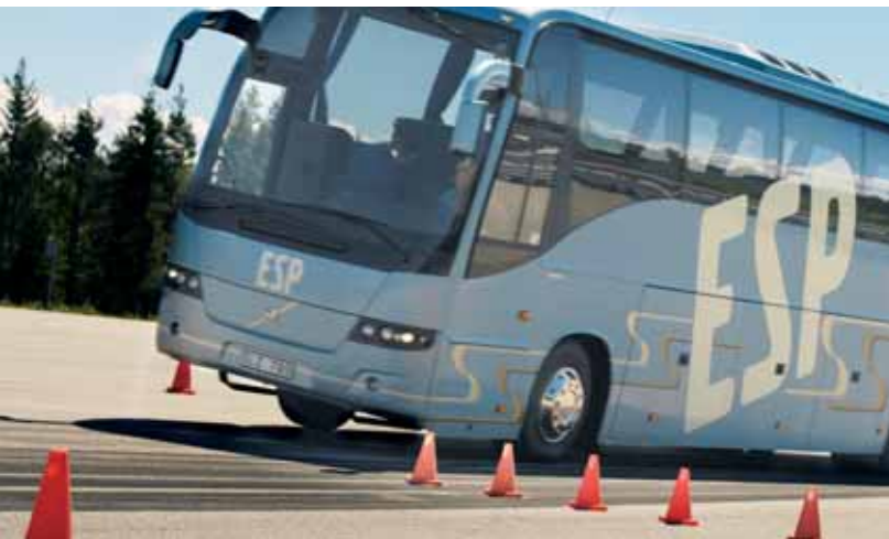
Electronic Stability Program (ESP) means much improved safety, and reduced risk of rolling over or driving off the road.
