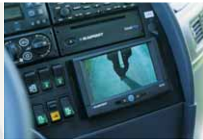
Cameras above the exits and rear of the bus are an excellent complement to the rear-view mirrors. The camera view is shown on a display on the instrument panel.
