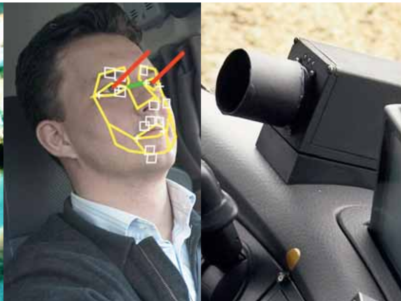
The driver's head movements, eye movements and blinking are monitored to prevent accidents due to drivers falling asleep at the wheel or being distracted.
