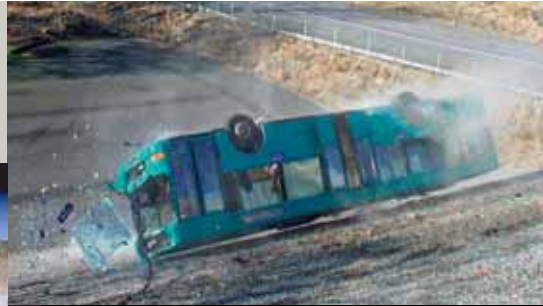
Full-scale roll-over test, which verifies the function of 3-point seatbelts
