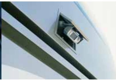
Cameras above the exits and rear of the bus are an excellent complement to the rear-view mirrors. The camera view is shown on a display on the instrument panel.
