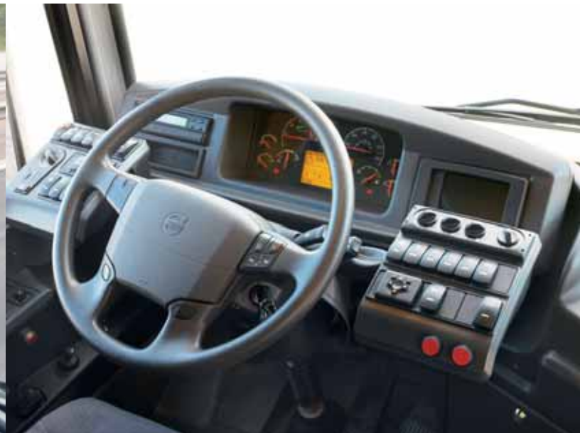
Volvo Buses' recently developed dashboard for city and intercity buses have controls logically grouped together by the side of the steering wheel.
