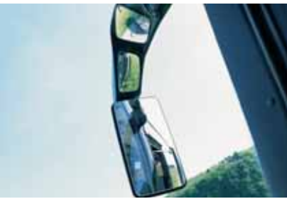
Three-piece rear-view mirrors provide very good visibility to the rear and the area immediately in front of the coach as well as by the front door and front wheels.
