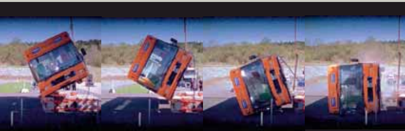
Full-scale R66 roll-over test, which evaluates the roof's strength. The bodywork should manage a roll-over without the roof collapsing.
