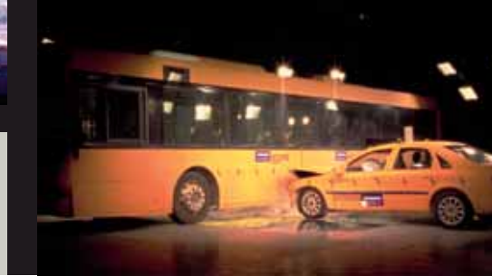
Full-scale side impact test to see the effects of a crash between a car and a city bus.
