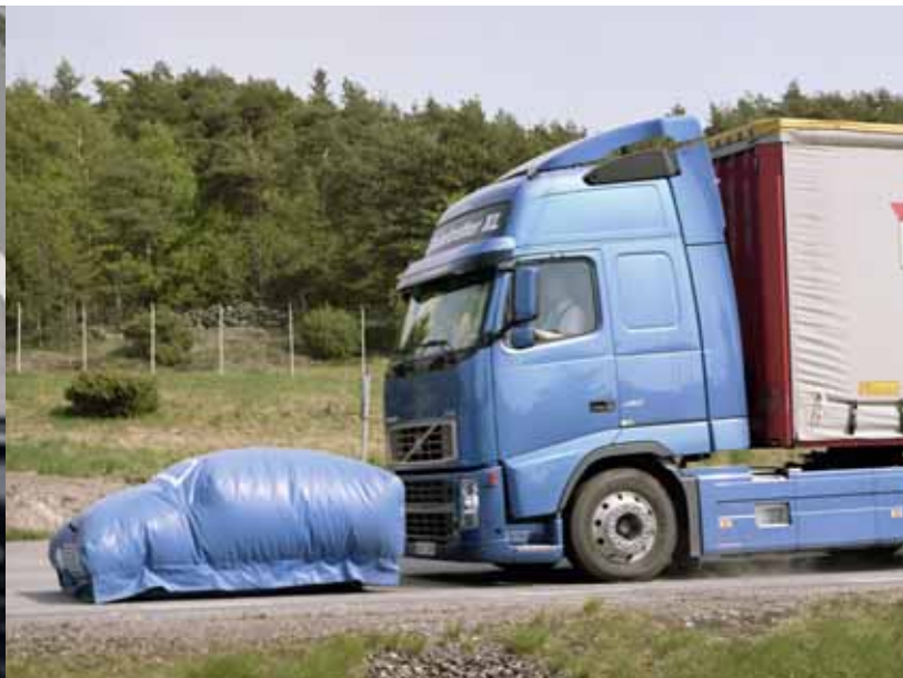
Adaptive Cruise Control is being developed for heavy vehicles in the Volvo Group. Shown here is a possible attribute: a truck's brakes are applied with full force when it risks driving into the vehicle ahead.
