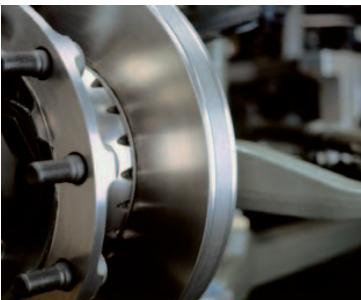
The brake disc is mounted on the hub via a patented spline-like joint allowing the disc to expand symmetrical.
