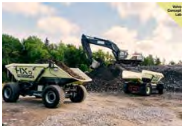
Two of Volvo CE's electric concept machines, the EX1 excavator and the HX2 hauler.
