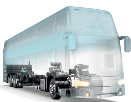
The B8L features an efficient driveline layout, without angle drive, which notably reduces fuel consumption and interior noise. The layout also allows larger free floor space for the passengers.
