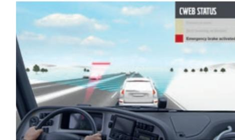
**CW-EB, Collision Warning with Emergency Brake**, detects vehicles in front and warns the driver when there is a collision risk. If the warning is ignored it is escalated and first followed by gentle braking, and then by emergency braking with maximum retardation.
