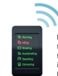
**I-Coaching** helps the driver to drive more safely, fuel efficiently and comfortably. It provides instant feedback on parameters such as over-revving, excessive idling, over-speed and harsh braking or cornering, helping the driver improve performance.
