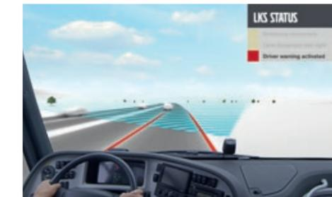
**LKS, Lane Keeping Support**, monitors the lane markings and alerts the driver when the risk of an unintentional lane departure is identified. The warning is given as a vibration in the seat, or as an acoustic signal.
