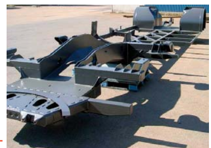
Prototype frame for Volvo Bus bi-articulated buses.
