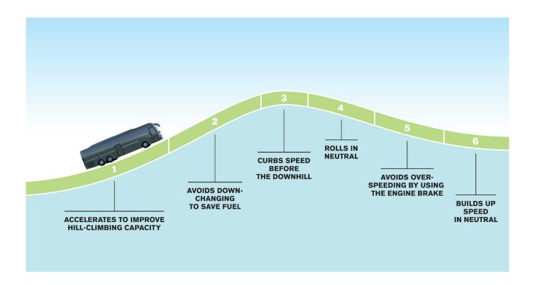
I-See is an advanced system that learns the topography of the road while you drive, helping you save up to 2.5% of fuel the next time you drive on the same road. In addition, the driver benefits from a more intuitive and comfortable driving sensation behind the wheel when driving with cruise control.
