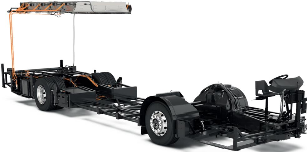
The Volvo BZL Electric single deck chassis offers outstanding flexibility for safe and efficient bodybuilding. Wheelbase and overhang can be adapted to fit each customer's requirements.
