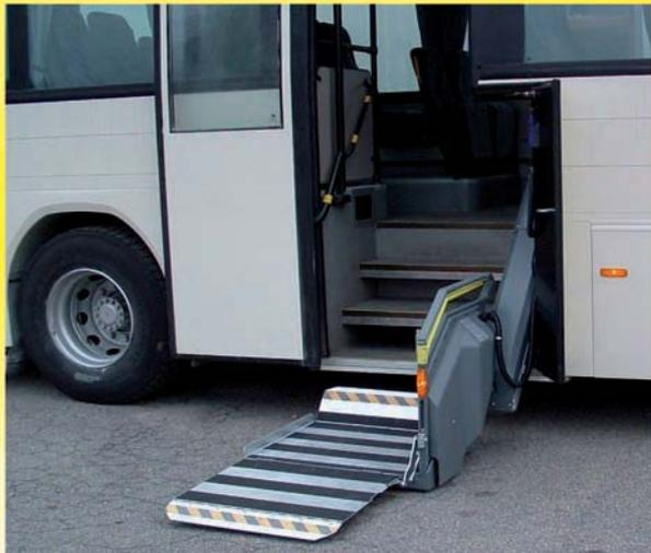
The TRPL-300 manufactured by Swedish U-Lift AB is the most well-known wheelchairlift for citybusses and coaches. Fully automatic operation makes it convenient and safe to use. Large liftplate with motorized roll-off-stops. Electrohydraulic operation with emergency system. Lifting heights up to 1500 mm. Meets European liftnorms.
