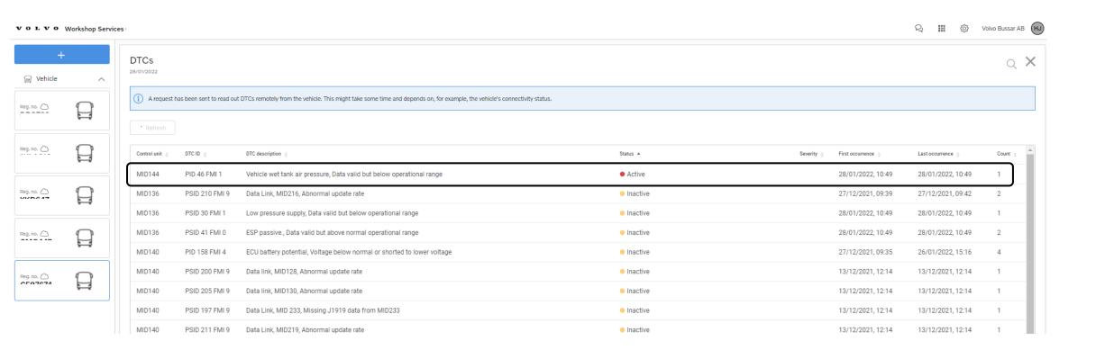
You can use the DTC library to find more information about the DTC's. Some DTC's have additional information about possible fault tracing. There are three ways of searching for the fault codes depending on what model and technical generation of the TGW.
