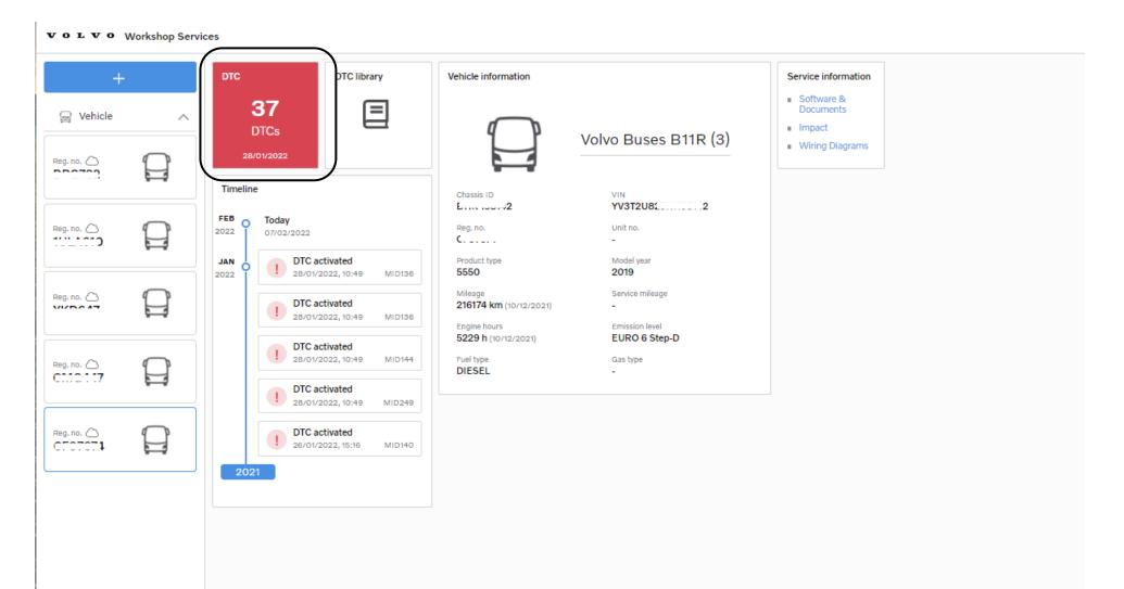
The list of fault codes, status and information about first and latest occurrence + how many times the fault occurred.
