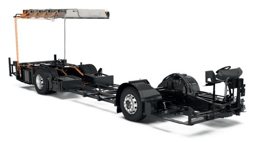
The Volvo BZL Electric single deck chassis offers outstanding flexibility for safe and efficient bodybuilding. Wheelbase and overhang can be adapted to fit each customer's requirements.
