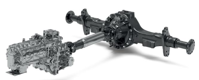
The all-Volvo driveline is available with single or dual motors. The propeller shaft concept makes for swift maintenance and improved comfort.
