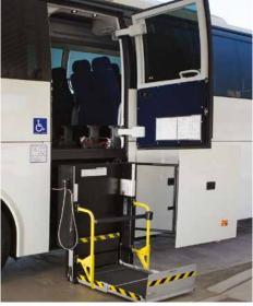
The under-the-floor wheelchair lift is invisible when not needed but easy to use as necessary. This compact lift has a durable steel construction for years of trouble-free operation, and meets all Americans with Disabilities Act (ADA) requirements.
