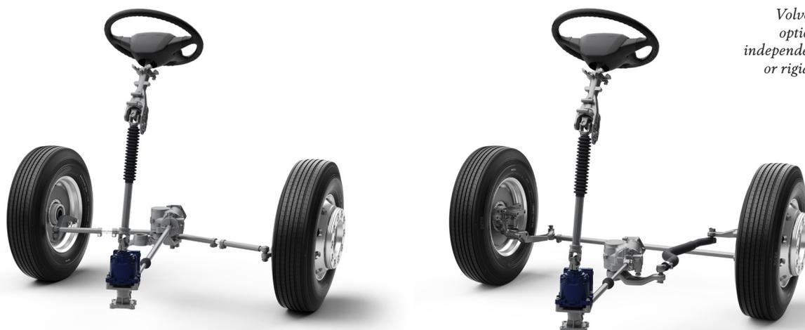
*Volvo Dynamic Steering is an option for vehicles with either independent front suspension (left) or rigid front suspension (right).*
