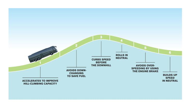
I-See is an advanced system that learns the topography of the road while you drive, helping you save up to 2.5% of fuel the next time you drive on the same road. In addition, the driver benefits from a more intuitive and comfortable driving sensation behind the wheel when driving with cruise control.
