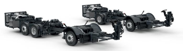
The Volvo B11R can be specified with features, such as Dynamic Chassis Lowering, the I-See fuel-saving feature and the unique Volvo Dynamic Steering.
