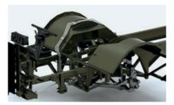
**Front suspension B11R** Rigid or independent front suspension is available, offering excellent comfort and handling along with a tight turning circle.
