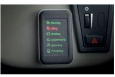
I-Coaching for smarter driving I-Coaching assists the driver in driving more safely, fuel-efficiently and comfortably. It gives instant feedback on vital parameters, helping the driver improve performance.
